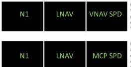
Example of FMA annunciations during a climb in **VNAV mode**. In this case, VNAV SPD indicates that the auto-flight system is following the FMC-programmed speed profile. N1 indicates that the auto-throttle system is commanding a set engine speed limit and LNAV (lateral navigation) indicates that the auto-flight system is following a programmed lateral track.
